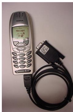
Fig.3. – Nokia 6310i to find a cable that matched the compressed serial output of the Nokia 6310i cell phone. The cable chosen was the Nokia DLR-3P serial cable, which has a
